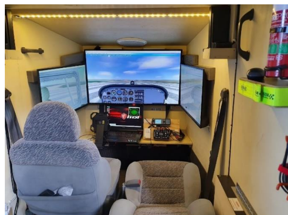
Illustrations: example of low-cost, portable (trailer-mounted), networked simulation facilities being used for COPAR training in Australia.
