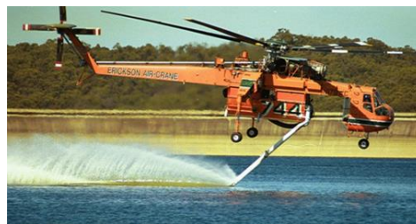
Illustration: example of super-heavy helicopter, Erickson S64 Air Crane, seen here in scooping mode.
