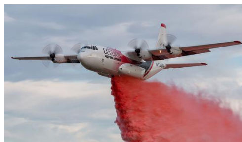
Illustration: C-130Q (equivalent to C-130H), large airtanker, with RADS dispensing system
